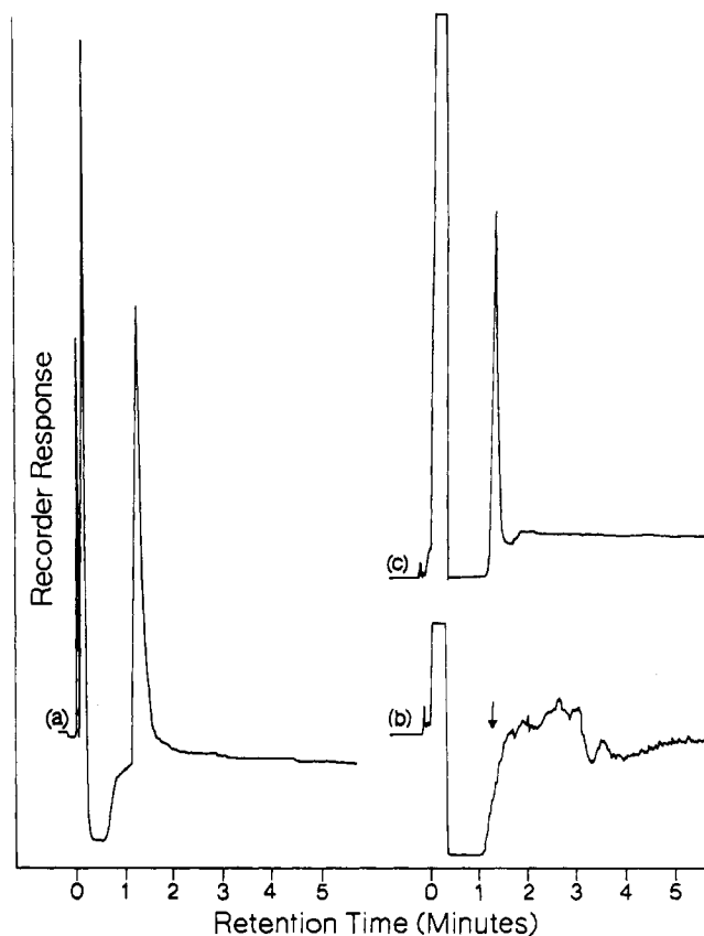
Figure 1. Gas chromatograms of (a) methomyl standard (10.61 ng), (b) untreated tobacco, and (c) untreated tobacco fortified with 2.00 ppm of methomyl. Instrument operating parameters are given in the text.
